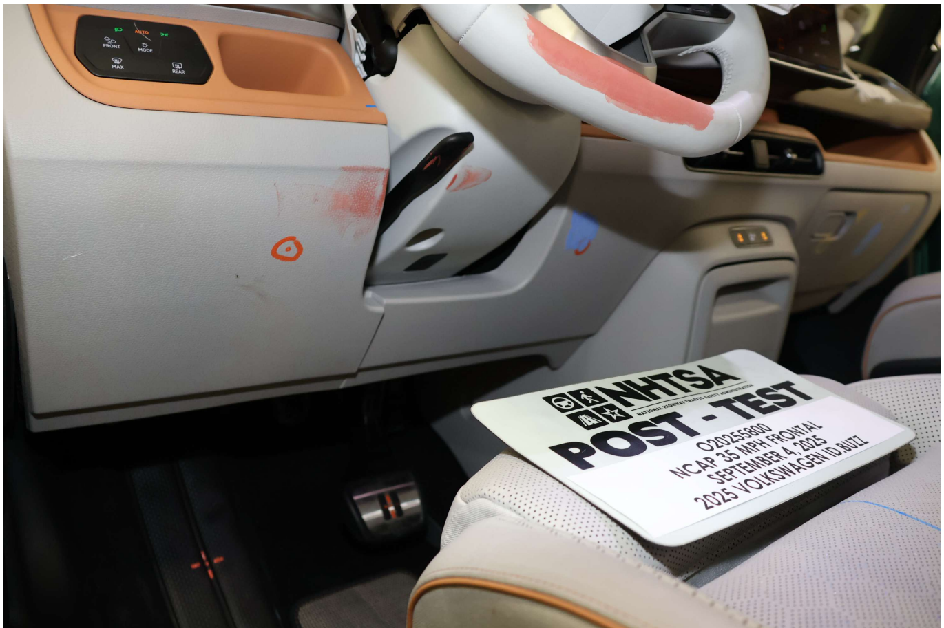
Photo No. 045 - Post-Test Driver's Side Knee Bolster
