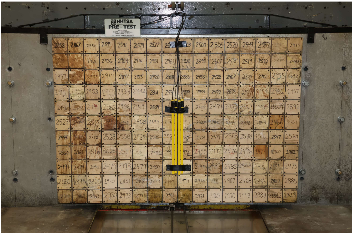
Photo No. 002 - Pre-Test Load Cell Wall
