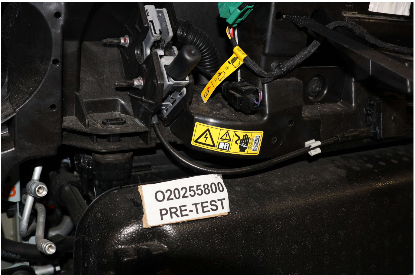
Photo No. 305-03 - First Responder Warning Label
