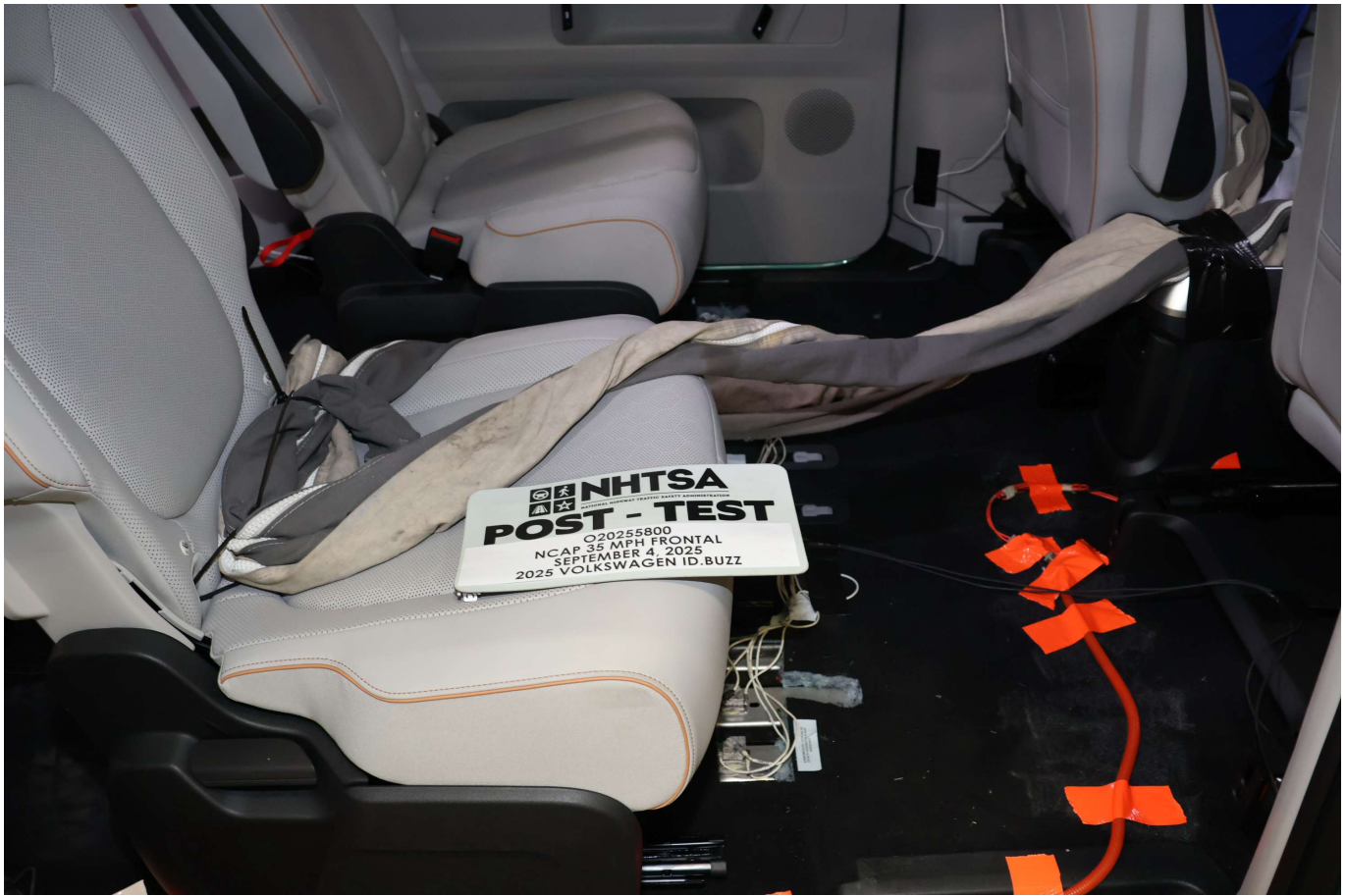
Photo No. 029 - Post-Test Dummy Cable Routing
