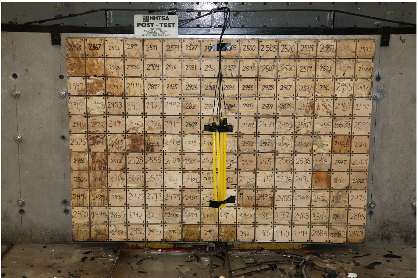
Photo No. 003 - Post-Test Load Cell Wall
